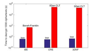
Figure 7: Comparison of time for decrypting 10<sup>3</sup> ciphertext tuples using the IRON implementation of IBE, ORE, 3DNF vs cryptographic implementations from pairings and mmaps respectively.
